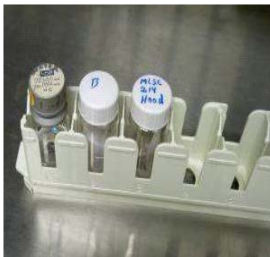
Plate 4 : Vials in Counting Rack.(Tri-carb- LSA 1000), CERT, ABU, Zaria.
