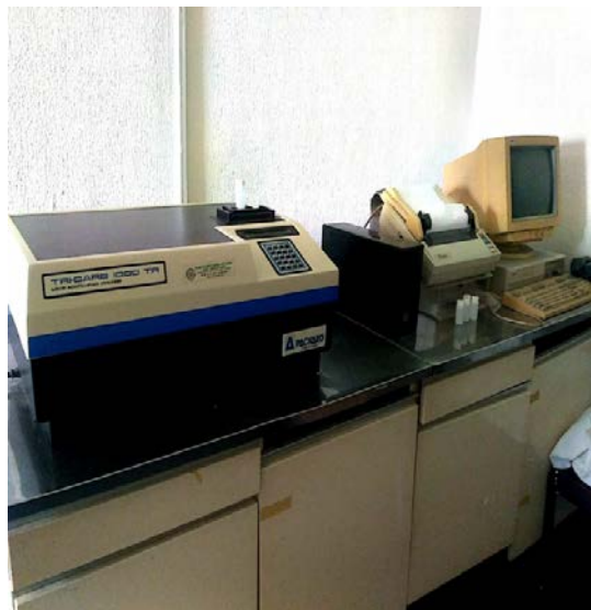
Plate 2: The Full Set of Liquid Scintillation Analyzer System (Tri-carb- LSA 1000), CERT, ABU, Zaria.
